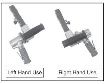
Figure 11. Left hand/right hand setup.
